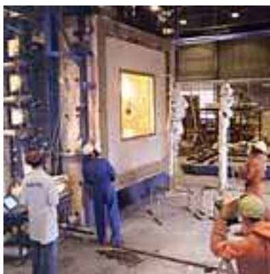
Figure 12: Large-scale structural fire resistance test of a window
