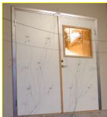
Figure 13: Insulation test of a door where thermocouples measure the temperature of the unexposed side during the heat exposure
