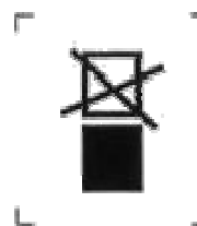
IBCs NOT capable of being stacked
