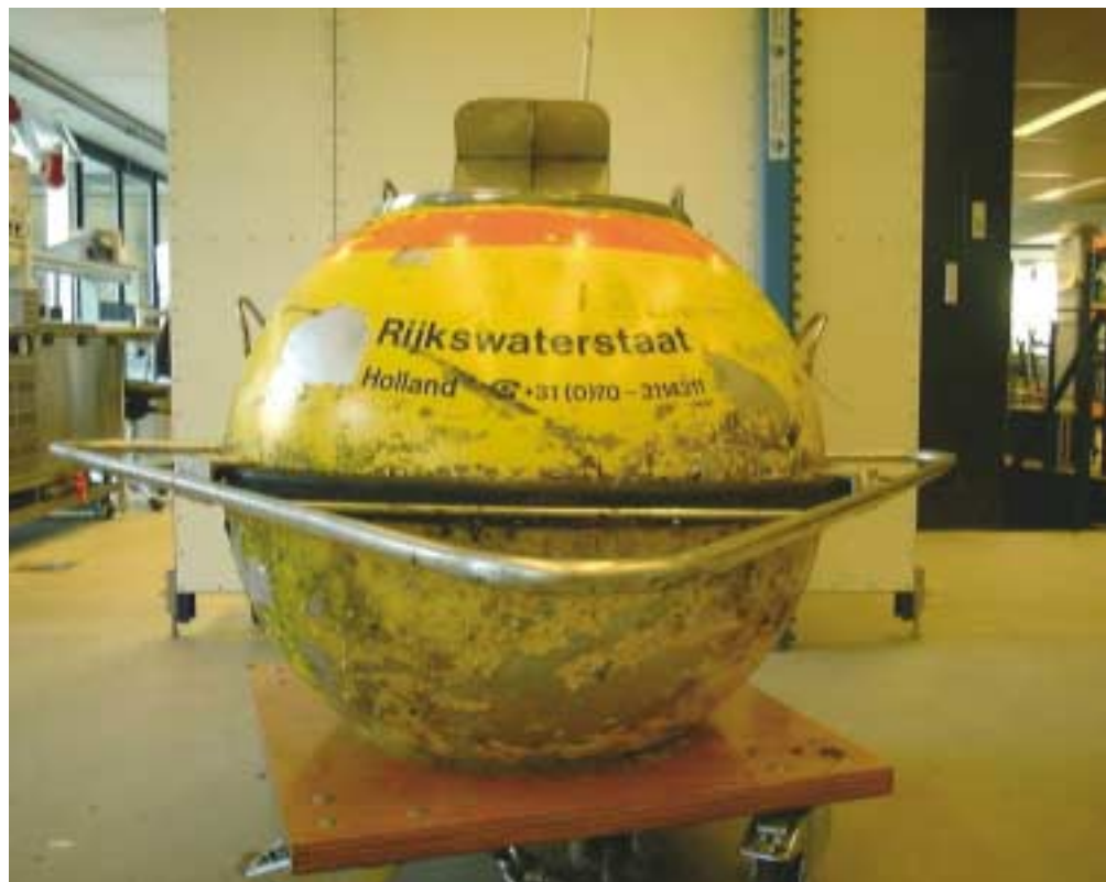
SON-meetboei in laboratorium ter controle (foto: RWS)
