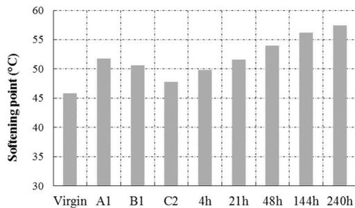
Fig. 2 Softening point results of virgin, field and artificially (RCAT) aged bitumen
