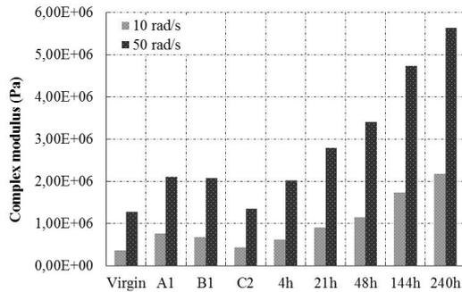
**Fig. 3** Comparison of complex modulus at an reference temperature of  $30^{\circ}\text{C}$
