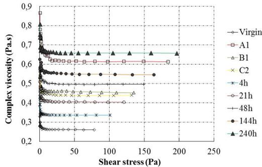
Fig. 4 Test results complex viscosity measurements at test temperature of 135°C
