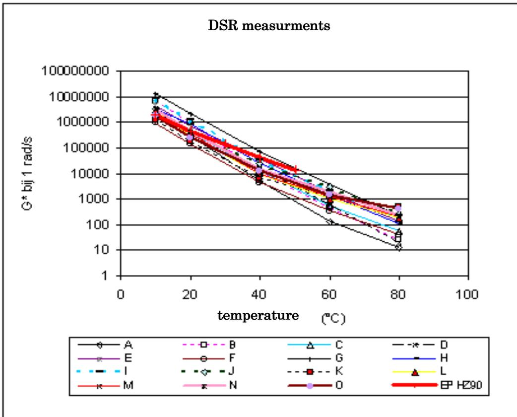
Figure 2: Results of DSR measurements of different binders used in PA.
