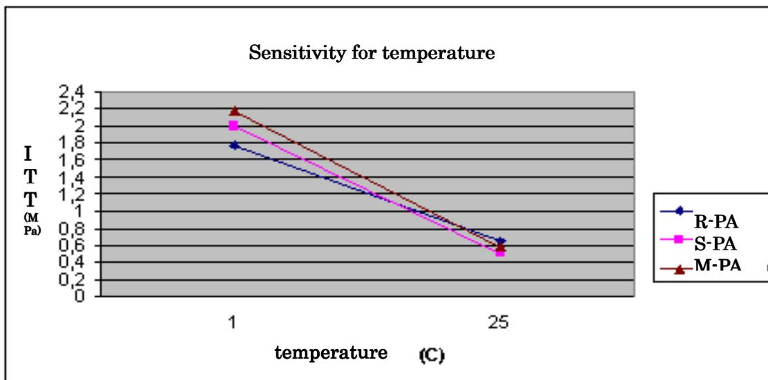
Figure 3: Results of temperature sensitivity of R-PA, S-PA and M-PA mixtures.
