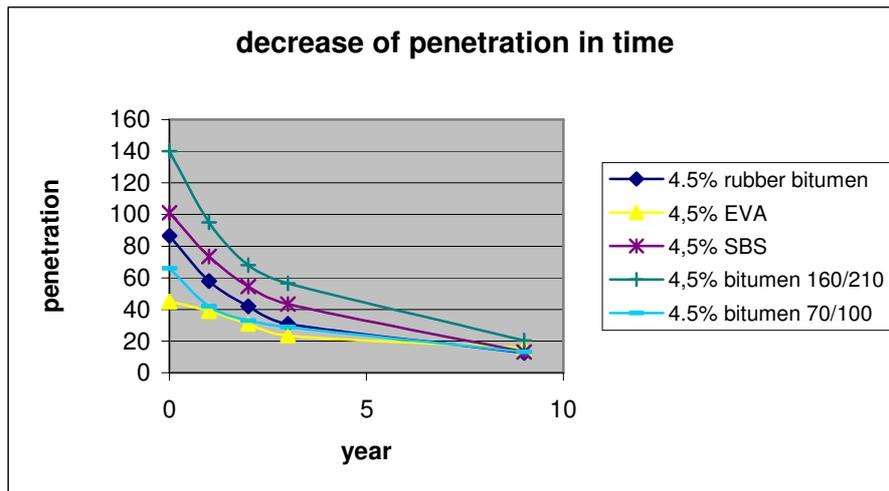
Figure1: Effect of binder ageing in time of PA mixtures with 4.2% binder in the mixture.
