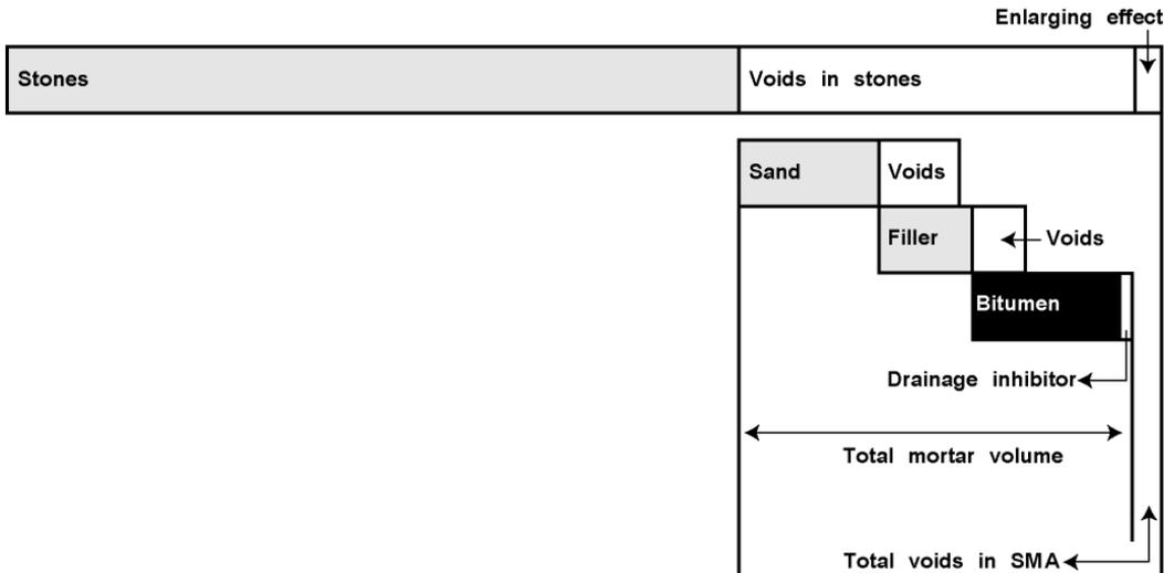
Figure 2: Volumetrically composition of SMA (schematically)
