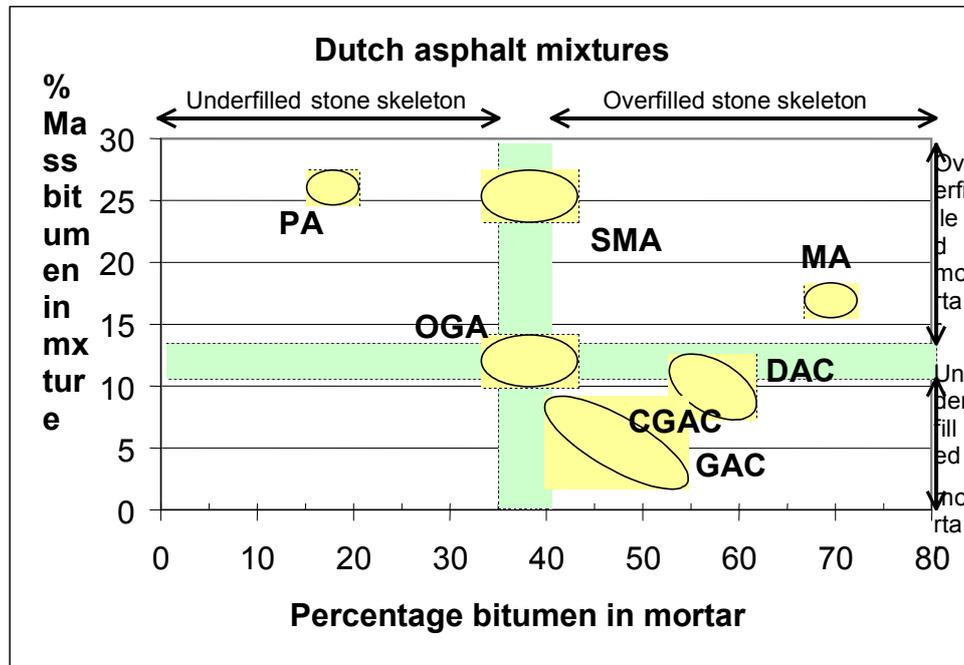
Figure 1: The volumetric characterisation of Dutch asphalt concrete mixtures
