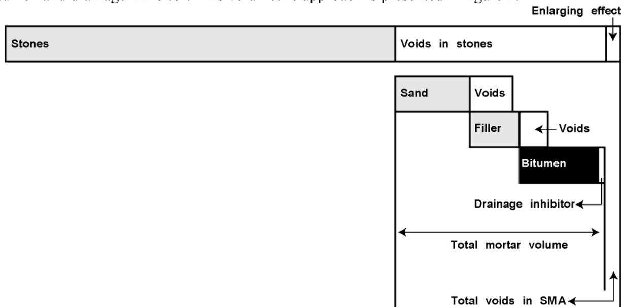
Figure 2: Volumetrical composition of SMA (schematically)
