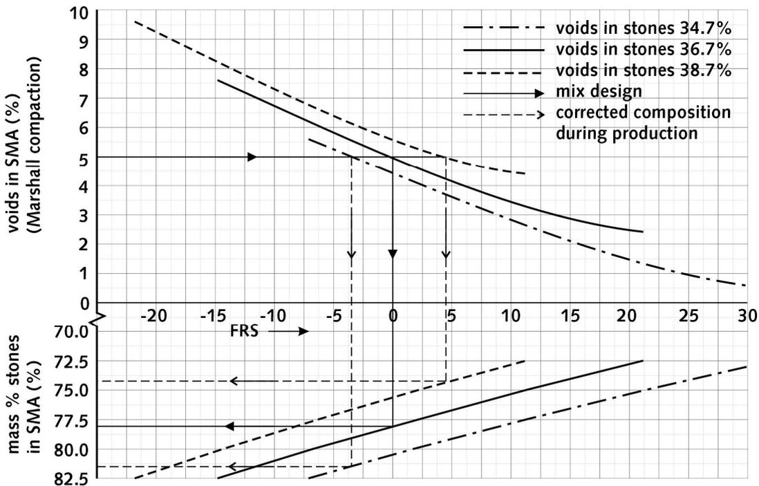
Figure 3: Graphical relation between air voids in the SMA, the  $FR_S$ -value and the known percentage crushed aggregates in the SMA
