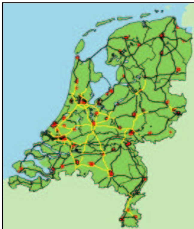
Figure 1. Signalised sections of the motorway network
