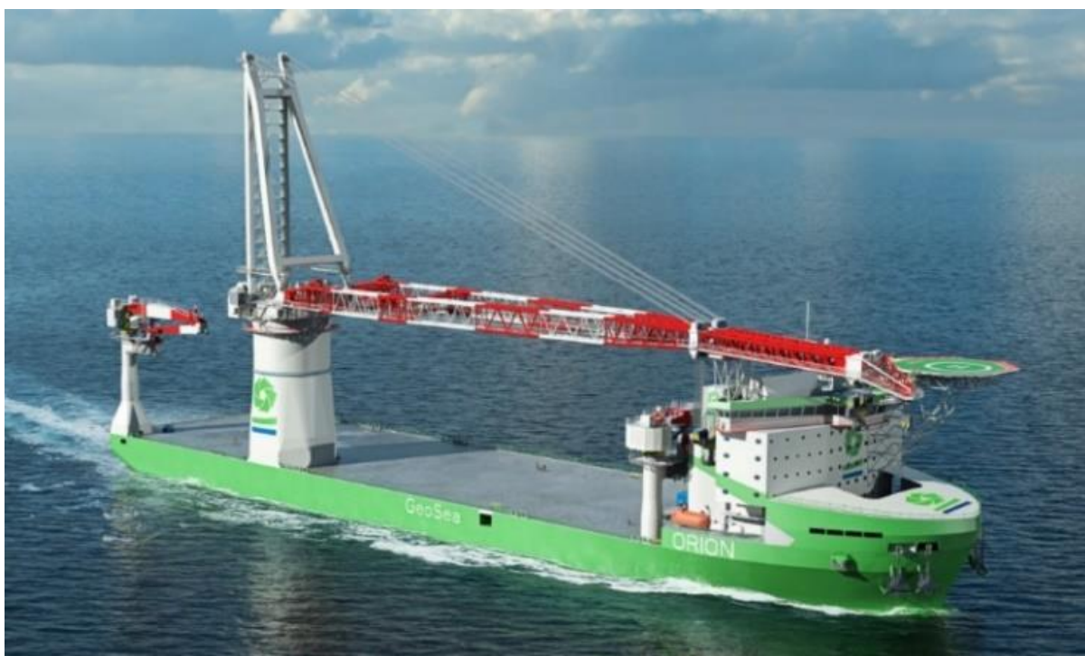
Figuur 5.1.2: Multipurpose offshore DP3 heavy lift vessel Orion
