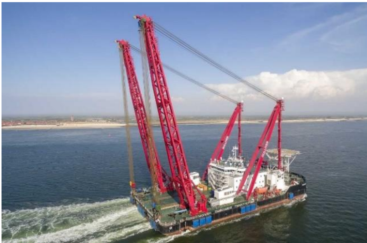
Figuur 5.1.1: Offshore DP2 Heavy lift vessel Gulliver
