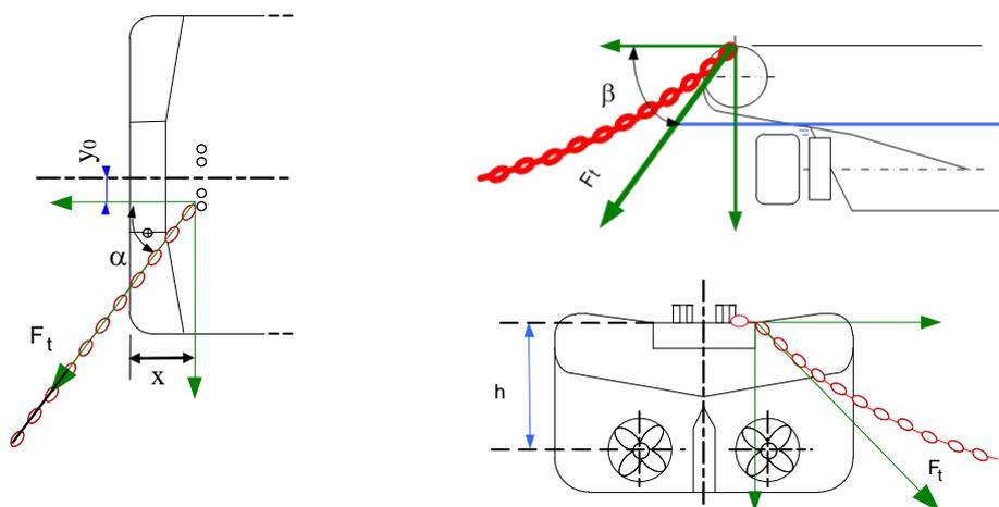
**Figure 2.7.2 – Diagrams showing the intended meaning of parameters  $\alpha$ ,  $\beta$ ,  $x$ ,  $y$  and  $h$ .  $F_t$  shows the vector of the applied wire tension."**
